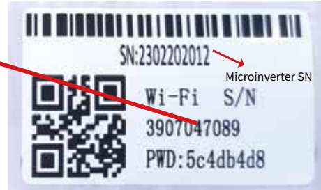
Microinverter SN: 2302202012 Built-in datallogger :3907047089
